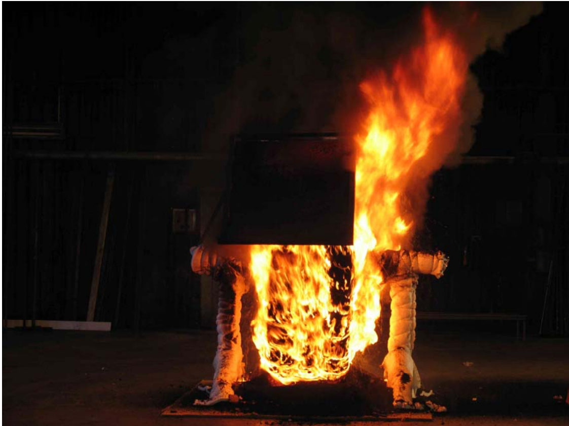
Figure 13 A photo taken 80 minutes from ignition. The heat release rate is about 2 MW.
