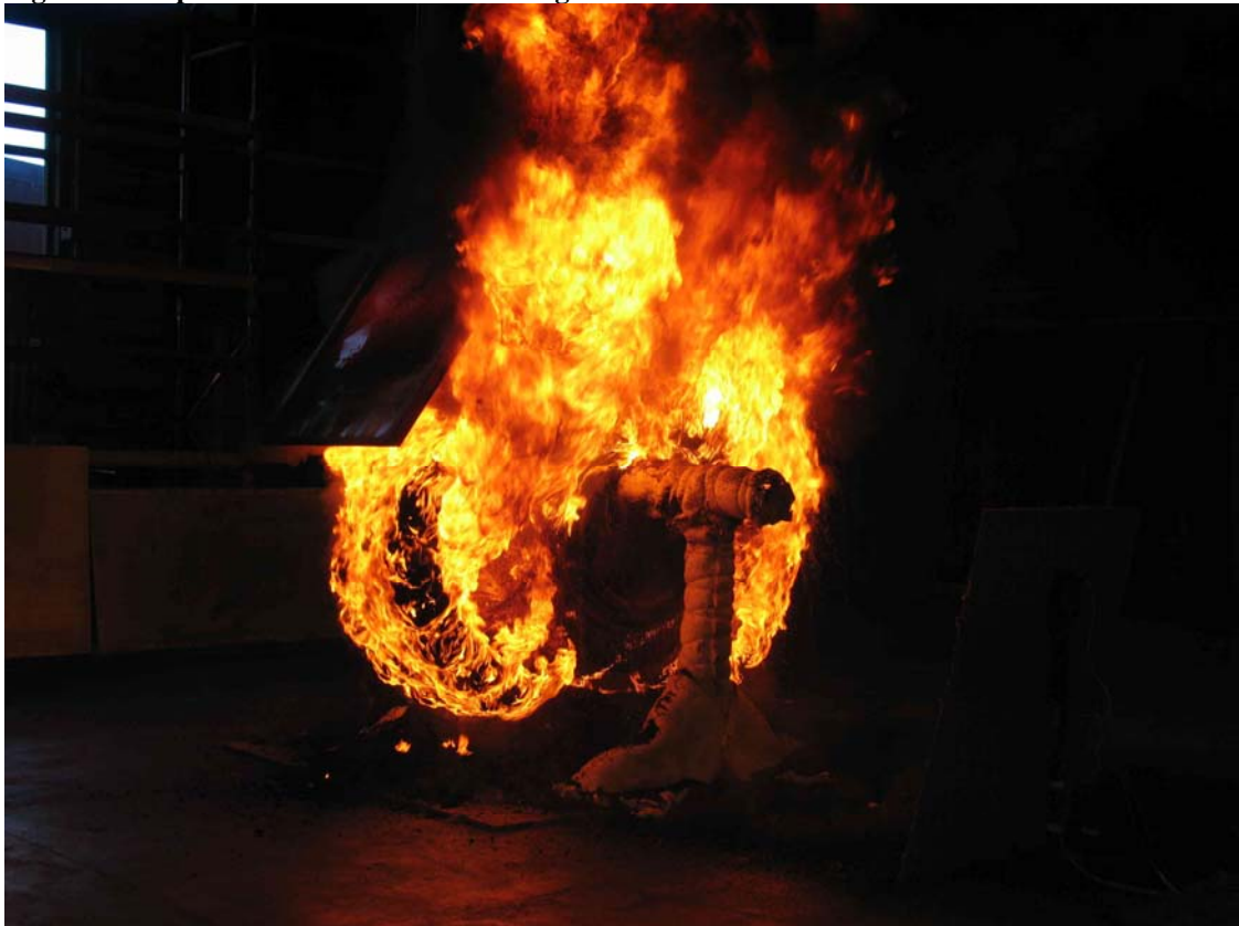
Figure 14 A photo taken 90 minutes from ignition. The heat release rate is about 3 MW. Notice that the tire is burning on two sides, i.e. on the inside and outside of the tire. This may explain the sudden increase in the peak heat release rate.
