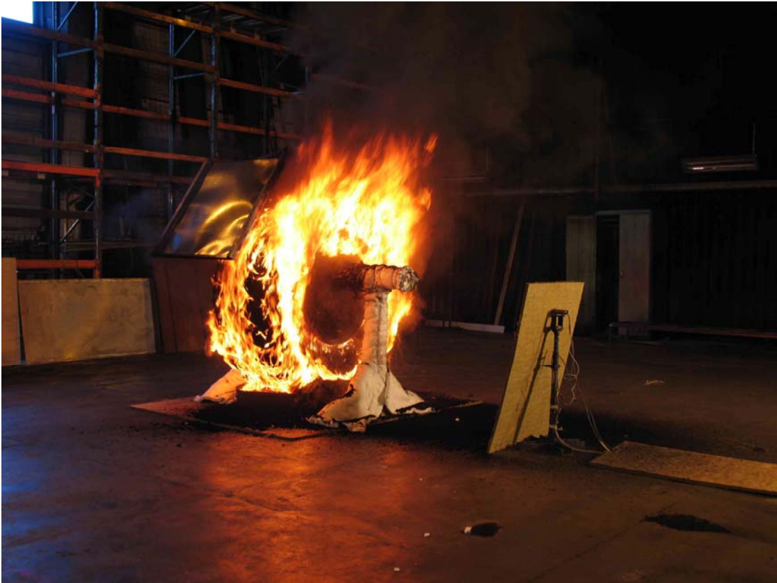
Figure 11 A photo taken after 60 minutes from ignition. The heat release rate is about 1 MW.
