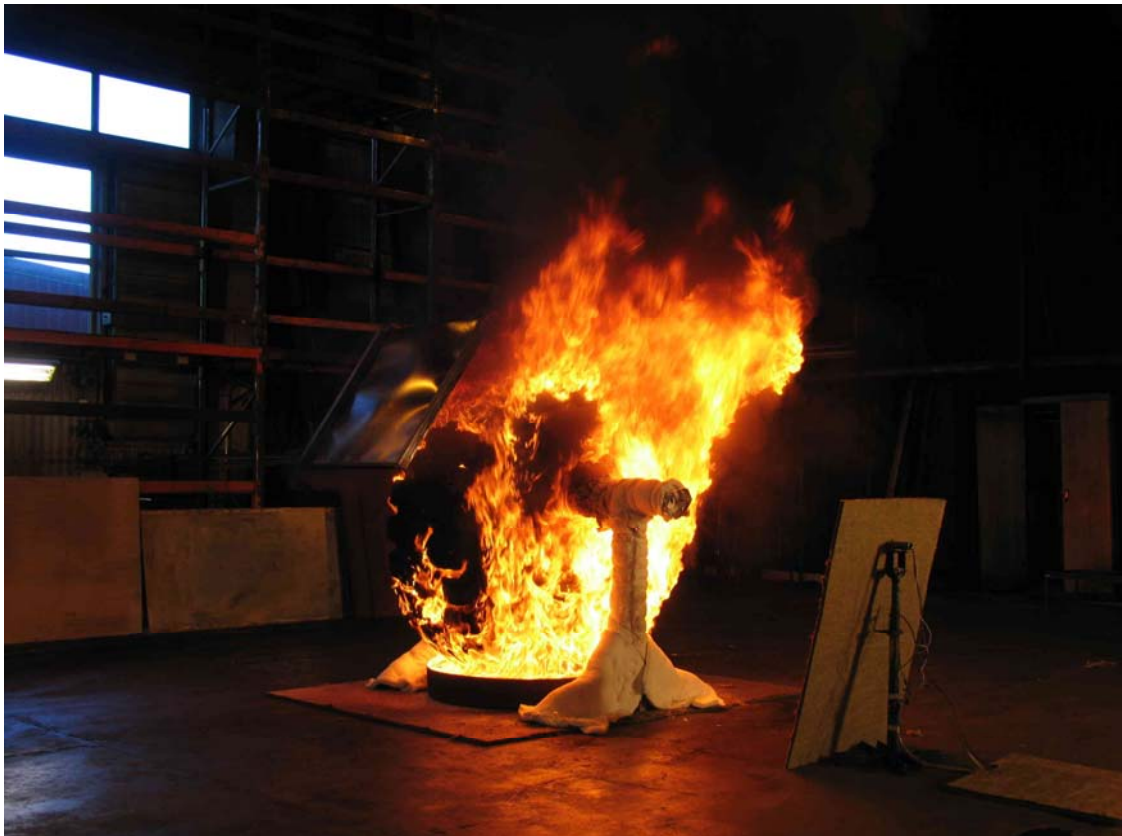
Figure 9 A photo taken after 4:16 minutes from ignition. The heat release rate is about 2 MWs. The peak heat release rate was 2.3 MW, and occurred after about 3 minutes from ignition.
