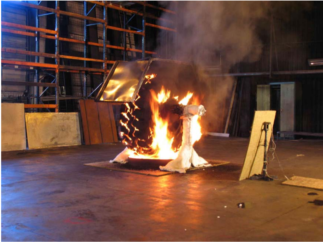
Figure 10 A photo taken when the first peak has reduced to only 0.4 MW after 20 minutes from ignition.
