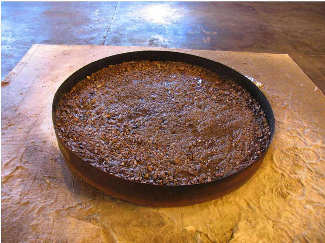
Figure 2 A photo of the diesel pan with loosely compacted gravel with stones sized from 0 – 18 mm. A total of 25 litre of diesel were poured into the 1.25 m diameter pan.
