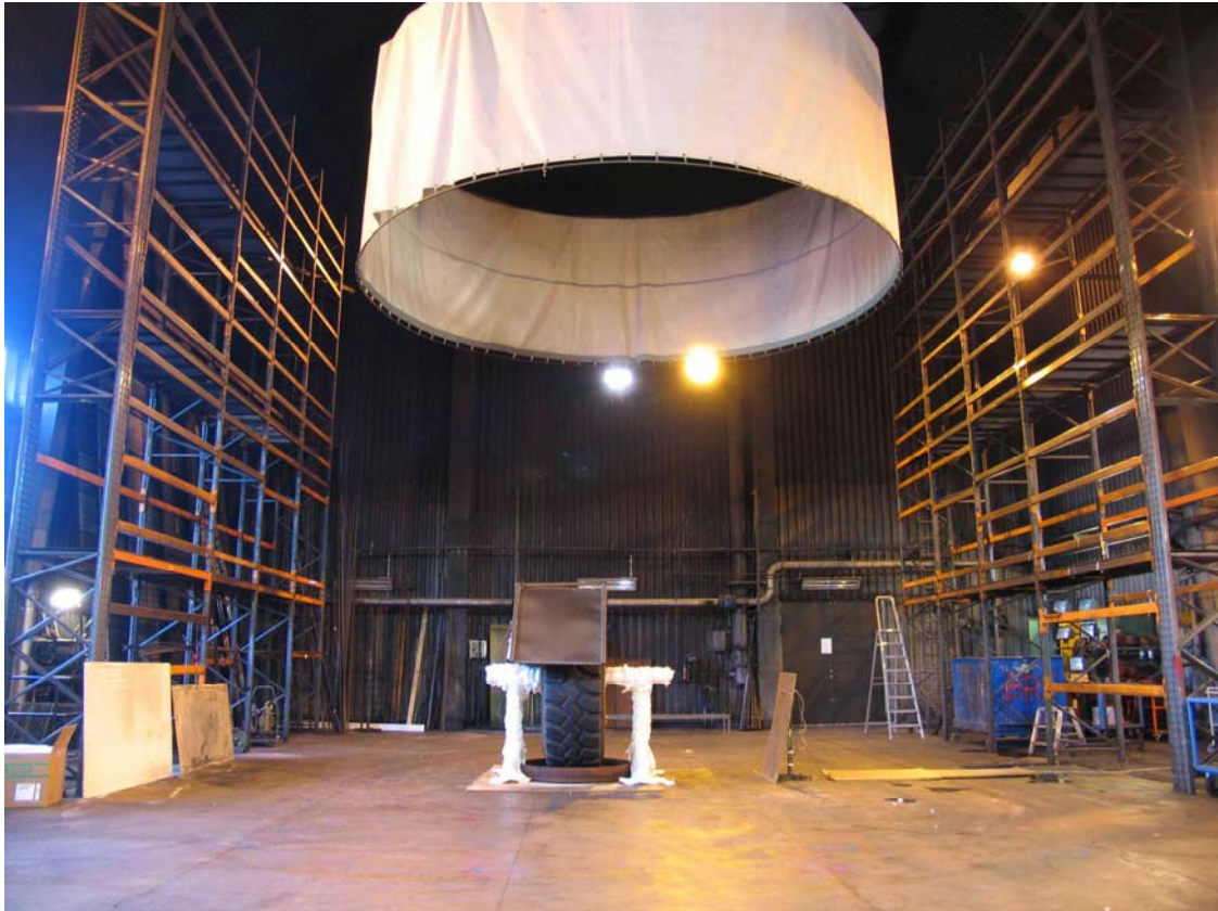
Figure 5 A photo of the test setup of the rubber tire prior to the test. The fire calorimeter is above the rubber tire and a Schmidt-Boelter heat flux meter is 1.5 m beside the tire.
